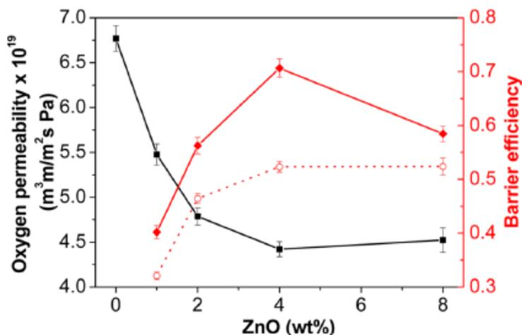
Figure 5. Oxygen permeability and barrier efficiency for water (solid diamonds) and oxygen (open circles) [51].
