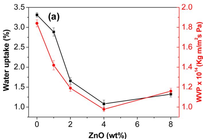
Figure 6. (a) water uptake and water vapor permeability (WVP) PHBV/ZnO nanocomposites as a function of ZnO content [51].
