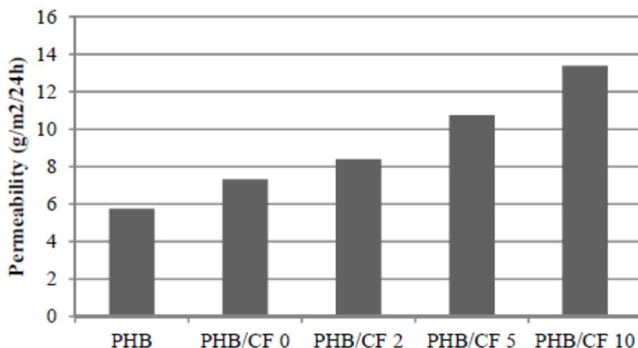
Figure 7. The effect of cellulose fiber over the permeability of the tested PHB composites and neat PHB [56].
